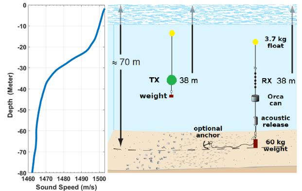
Fig. 3: Channel geometry of two nodes in the depth of 38 meters
