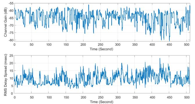
Fig. 5: Illustration of instantaneous variations of channels gain and RMS delay spread resulted from the statistical model
