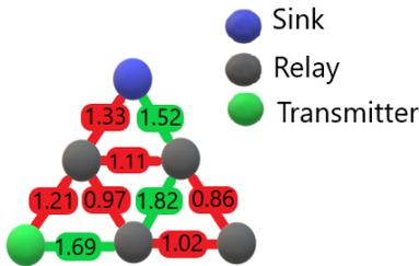
Fig. 10: Illustration of packet routing in network using channel quality
