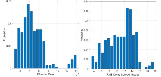
Fig. 9: Posterior PDF of the channel's gain and RMS delay spread
