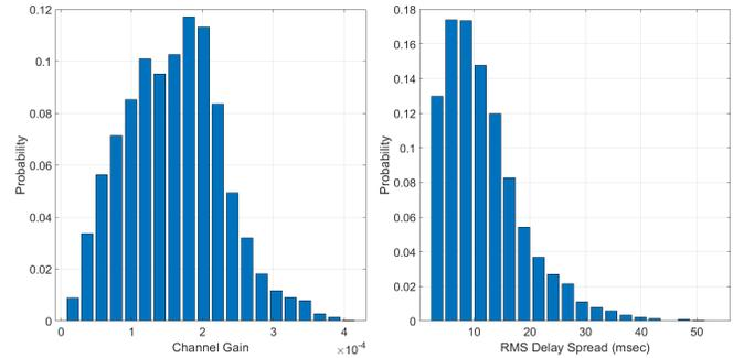
Fig. 8: Illustration of measured channel gain and RMS delay spread PDF during DalComms1
