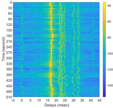
Fig. 4: channel impulse response of two nodes in depth of 38 meters
