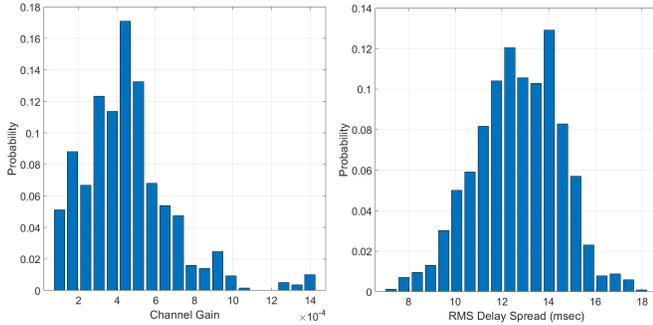
Fig. 6: PDF of channels RMS delay spread and channel gain from statistical model
